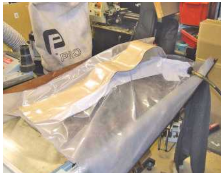
▲ Pic.14 Apply glue to the layers of veneer with a roller to get a smooth, even coat, then pop in the bag
